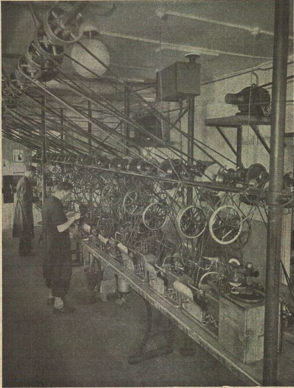
Working the jewels to the precise diameter.
